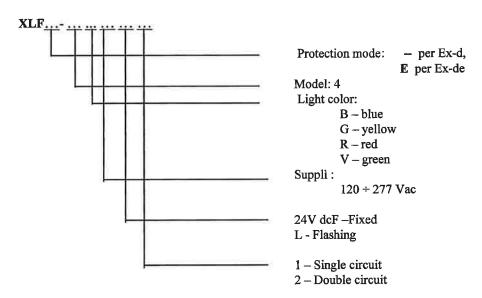
The XLF.. series equipments can be realized with protection mode "Ex de" by means of a "Ex-e" terminal box added on the ceiling fixture of the "Ex d" lamp compartment. The cable passage between the "Ex d" and the "Ex e" compartment is made by means a special certified bushing..
