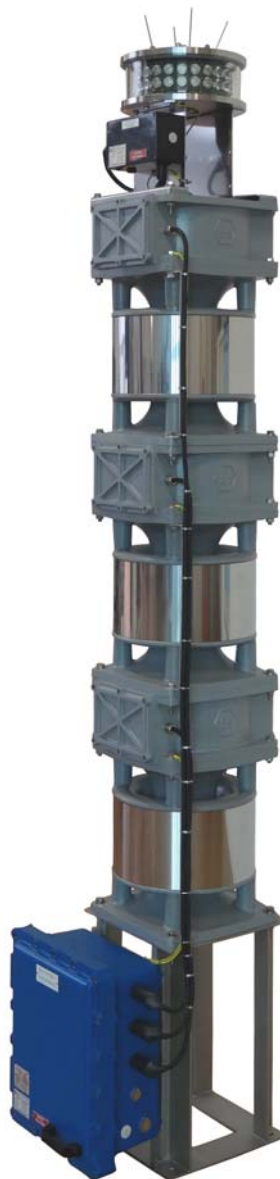
SICE NV-V3 MAIN FOG HORN 2 NAUTICAL MILE RANGE INCLUDING LOCAL CONTROL CIRCUIT ENCLOSED IN A Ex-d JUNCTION BOX AND TOP LED LANTERN
