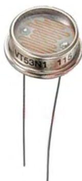
VT50N1 (OR EQUIVALENT) PHOTOCONDUCTIVE CELL SENSOR INSTALLED INSIDE ENCLOSURE
